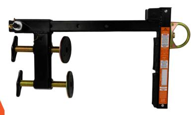
The Malta Dynamics Parapet Wall anchor was designed to be used on flat roofs that are surrounded by a parapet wall. This anchor is fully adjustable and can be installed on wall thicknesses from 2.36" all the way up to 14.1 inches. This anchorage device is nonpenetrating and requires no tools to install
